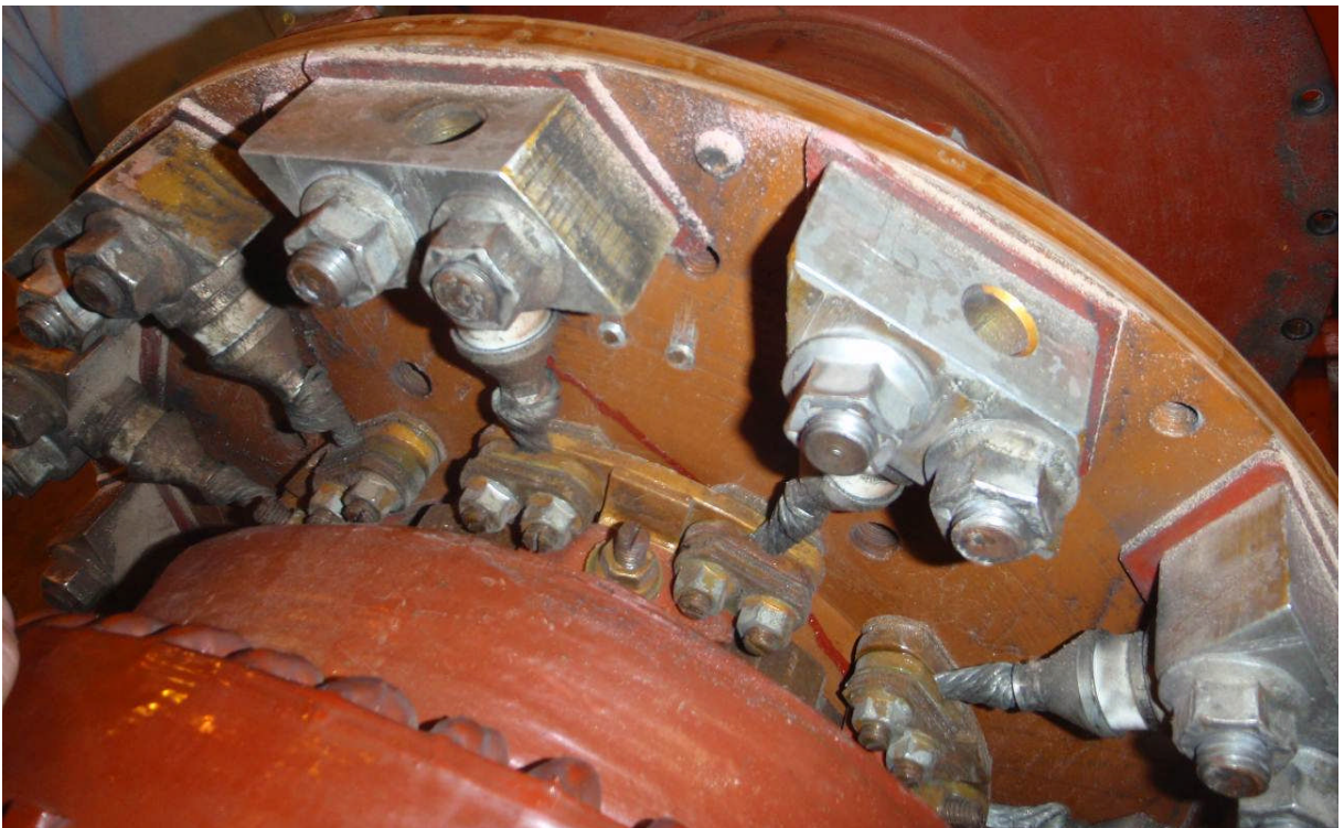
Figure 4: Diodes Found with Twisted and Deformed Flexible Connectors
