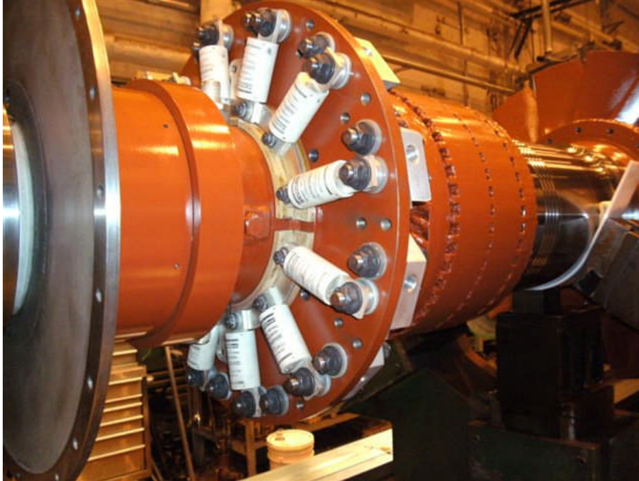
Figure 25. Installing Fuses on Diode Wheel
