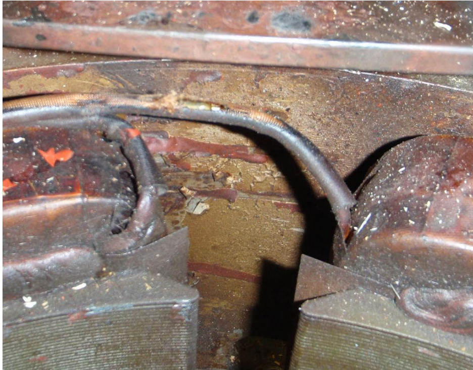
Figure 7: Cracked and Brittle Insulation
