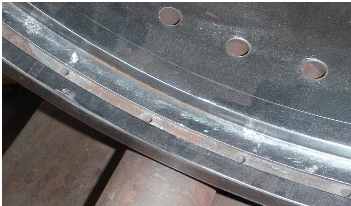
Figure 15: Aluminum on Retaining Ring Fit Area
