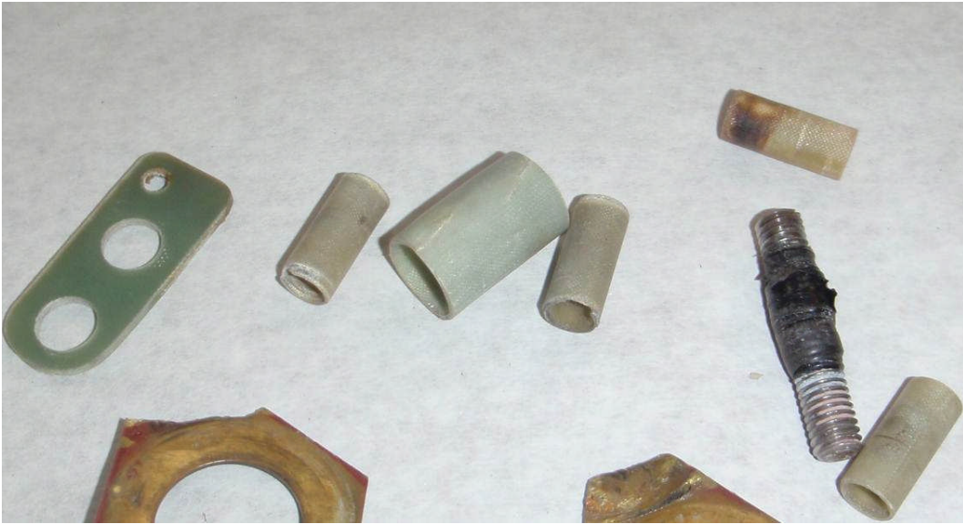
Figure 3: Worn Insulating Components
