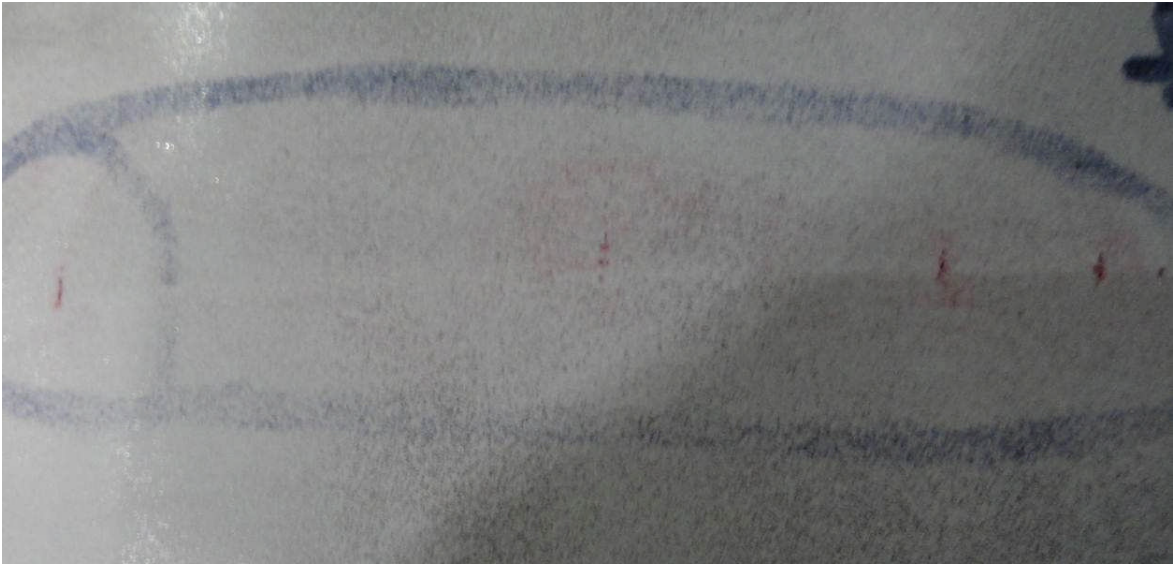
Figure 19: Dye Penetrant Test Indications on EE Retaining Ring
