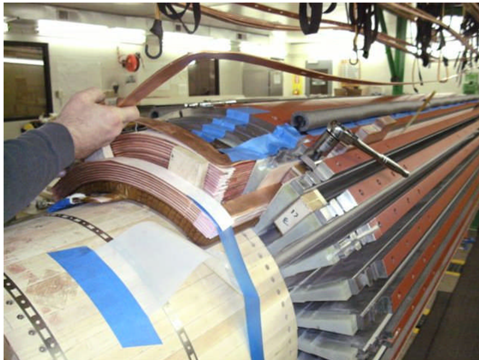
Figure 22: Initiation of Rotor Rewind Process
