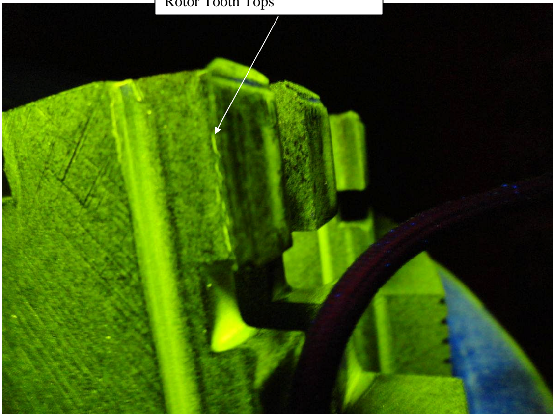
Linear Indications Found on Rotor Tooth Tops
