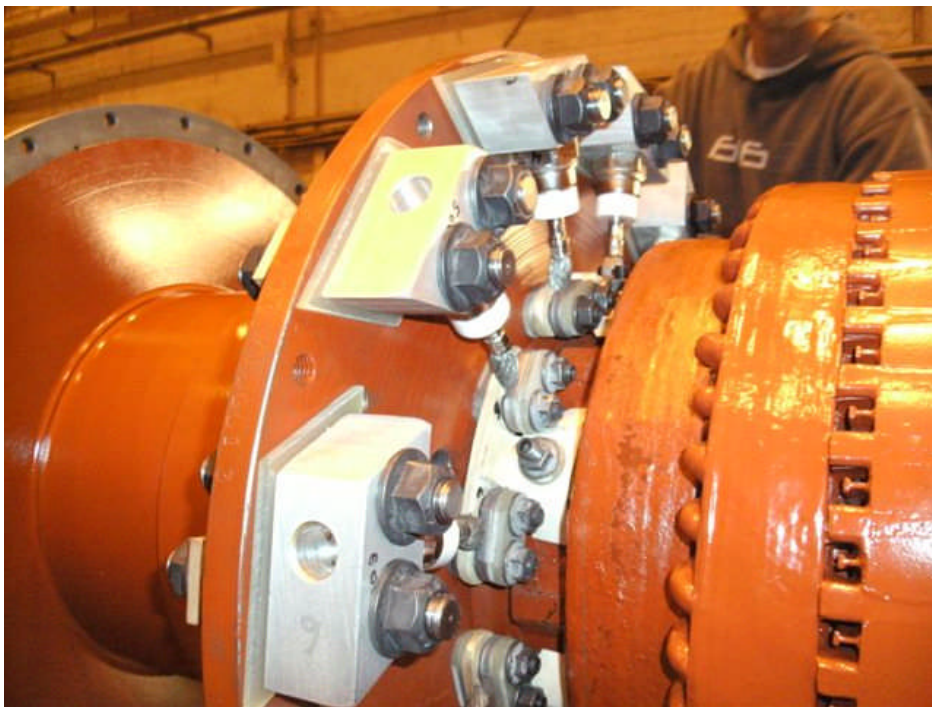
Figure 24. Installing New Diodes on Diode Wheel
