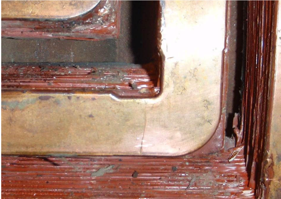
Figure 13: Crack Found on Top Turn of Coil 5, Exciter End
