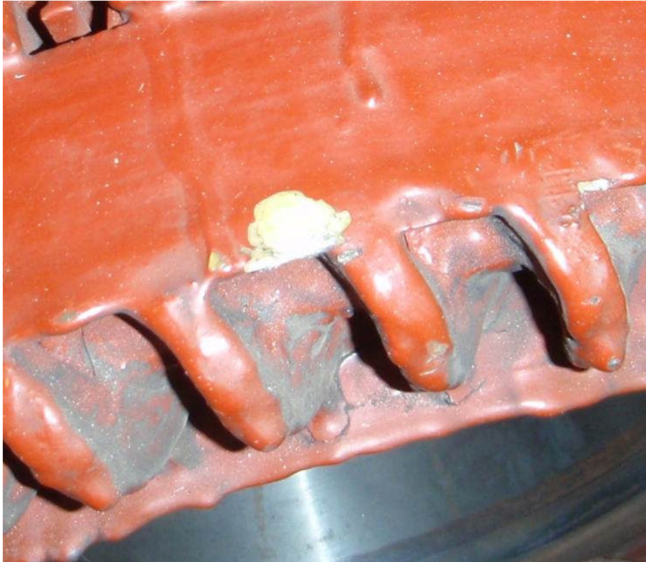
Figure 9: Minor Damage Found on Outboard Band
