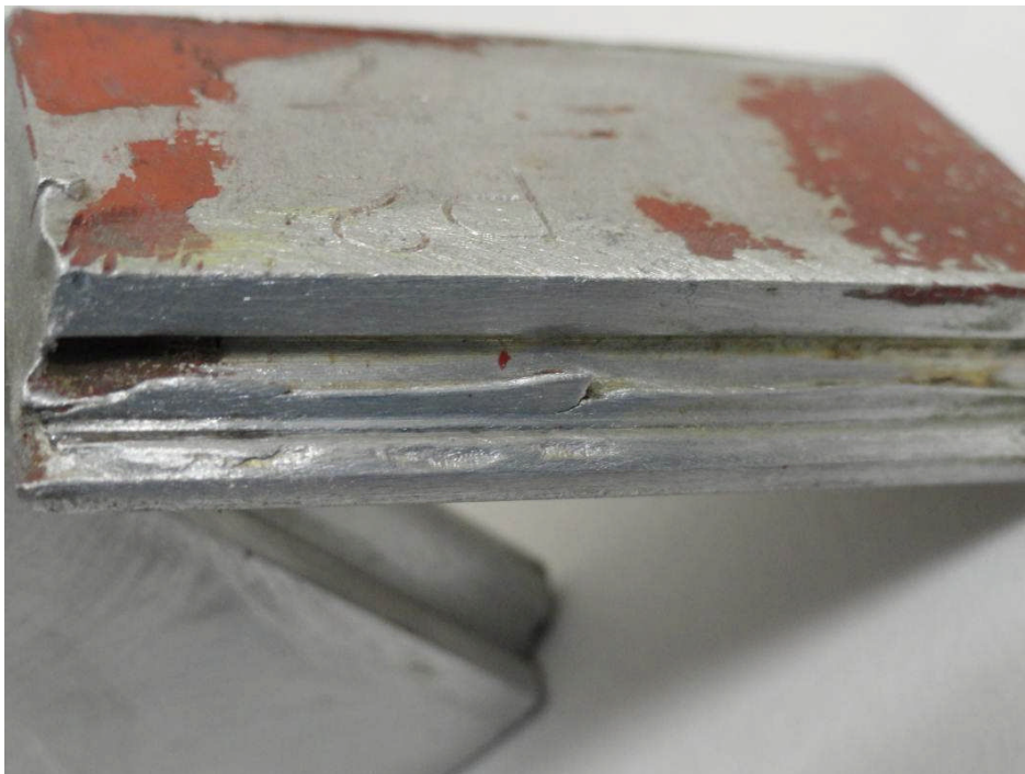
Figure 12: J-Lead Wedge in Poor Condition as found
