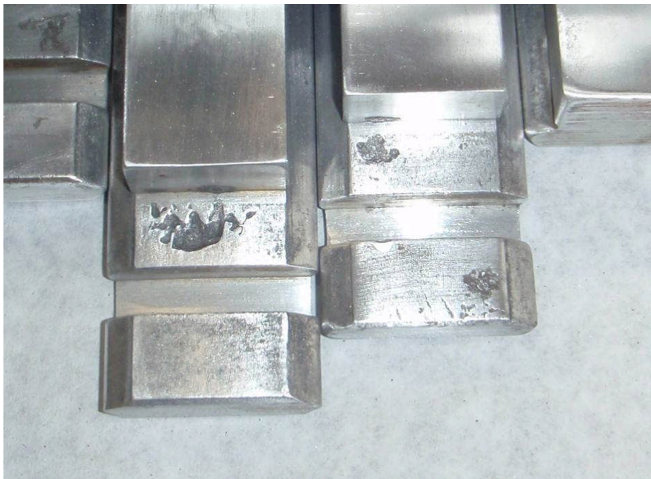
Figure 14: Arcing Damage to Slot Wedges
