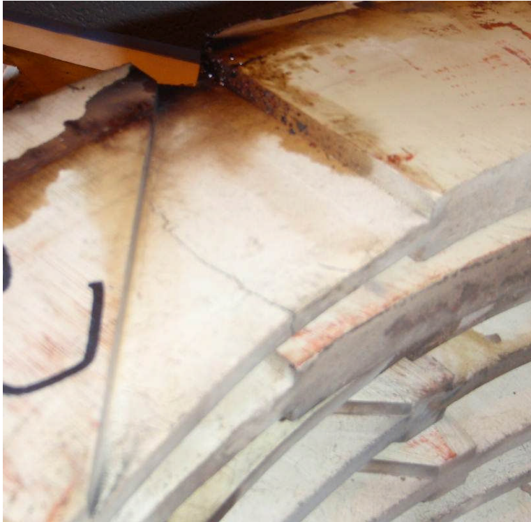
Figure 11: Cracking in End Winding Blocking
